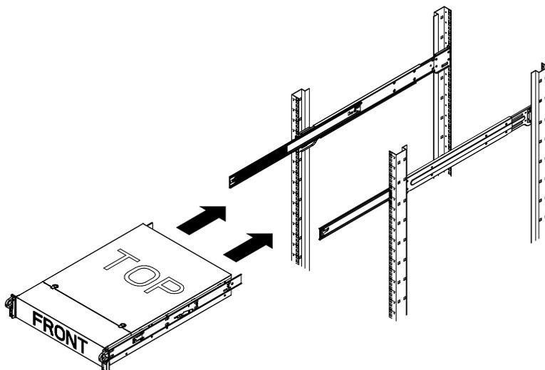
**To install the chassis in the rack:**
