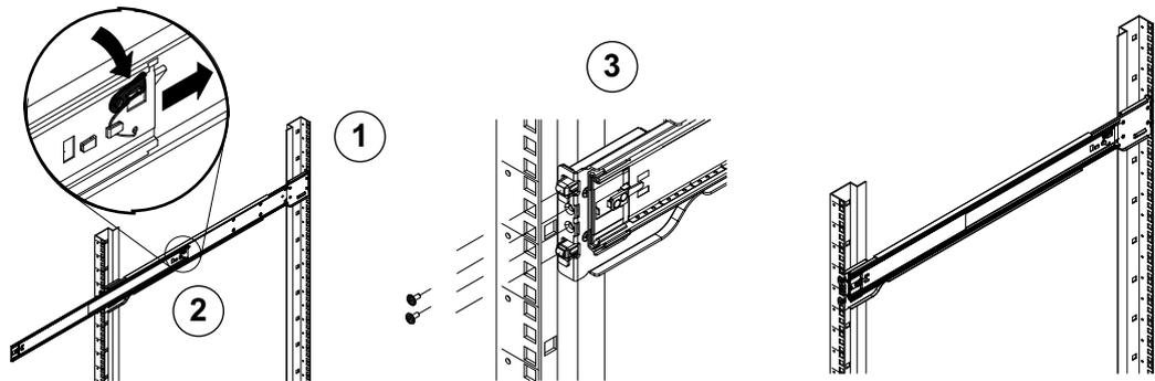
**To install the outer rails to the rack:**
