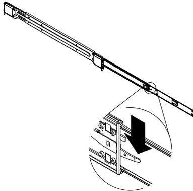
4. Separate the inner rail extension from the outer rail assembly.
