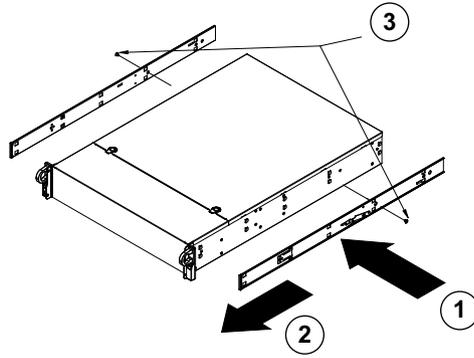
**To install the inner rails:**
