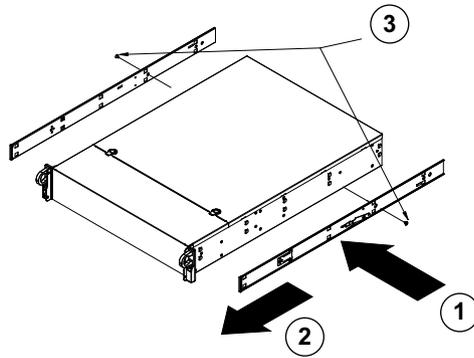
**To install the inner rails:**
