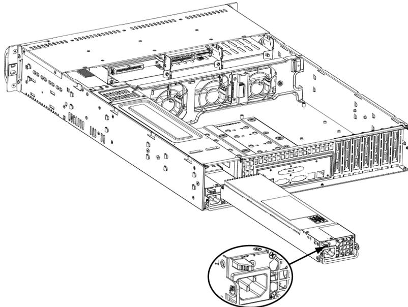
3. Pull the power supply out using the handle provided.
