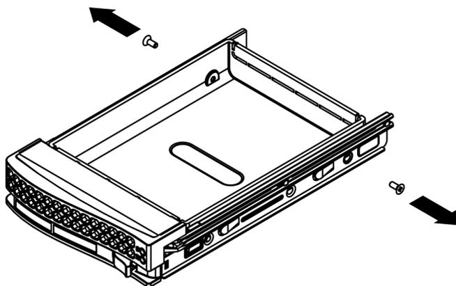
2. Remove the dummy drive from the hard drive carrier and place the hard drive carrier on a flat surface.
