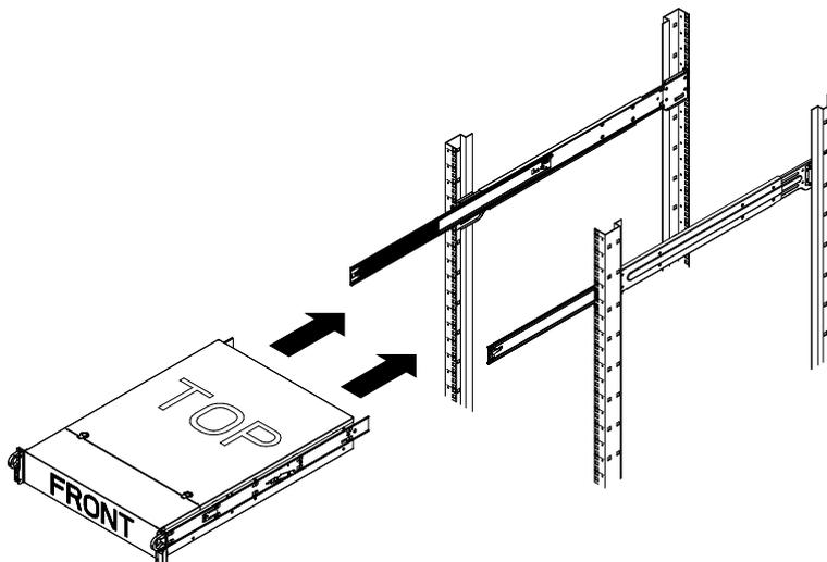
**Installing the chassis in a Telco type rack**
