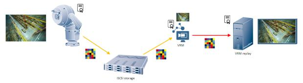
Only replay clients that are known by the camera (by means of a certificate containing the client's public key) at the time of recording can decrypt the video footage. If a workstation is added to the system, only the video recorded after the workstation is added will be available for decryption by the new workstation. Existing workstations have access to the historical recording as well.
