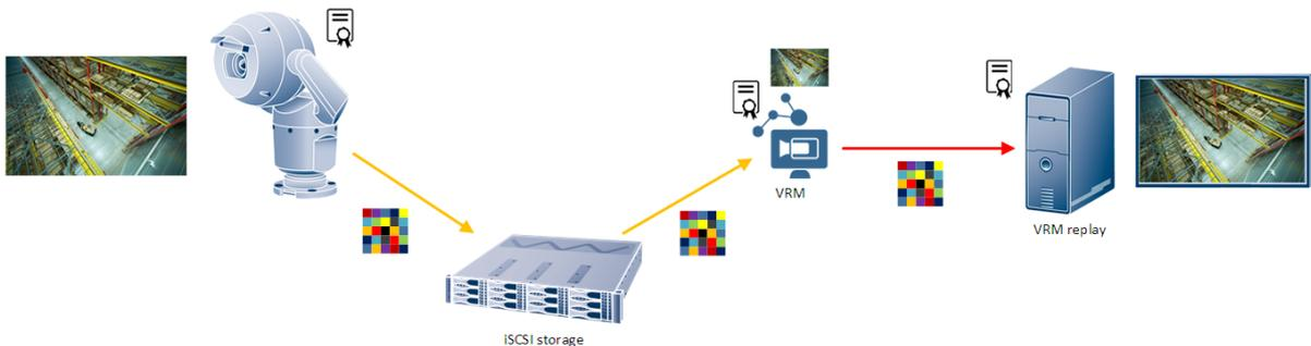
Only replay clients that are known by the camera (by means of a certificate containing the client's public key) at the time of recording can decrypt the video footage. If a workstation is added to the system, only the video recorded after the workstation is added will be available for decryption by the new workstation. Existing workstations have access to the historical recording as well.
