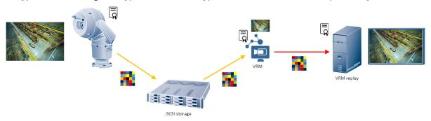
Only replay clients that are known by the camera (by means of a certificate containing the client's public key) at the time of recording can decrypt the video footage. If a workstation is added to the system, only the video recorded after the workstation is added will be available for decryption by the new workstation. Existing workstations have access to the historical recording as well.
