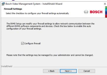
The firewall configuration dialog is a fixed step in the setup process and will allow automatic configuration of all required firewall settings to run BVMS.
