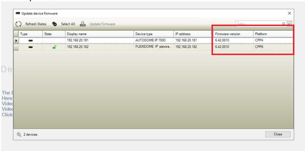
If the combined firmware package is used, multiple devices can be selected for a parallel upgrade. The upgrade speed depends on the network infrastructure. The Open dialog box is displayed.
