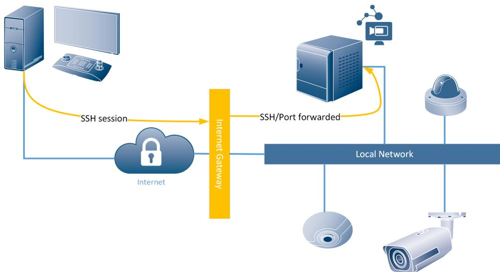
The SSH client is embedded into the BVMS Operator Client. The SSH service can be, optionally, installed on the BVMS management server. When using SSH tunneling, all BVMS related traffic is routed through the SSH service and this will therefore also create a single-point-of-failure in the system.
