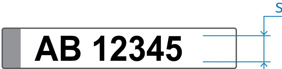
A character height of 16 pixels in the processed image is considered the optimal pixel density. The application can still recognize plates with smaller character heights, such as 10-12 pixels per character in non-noisy images.
