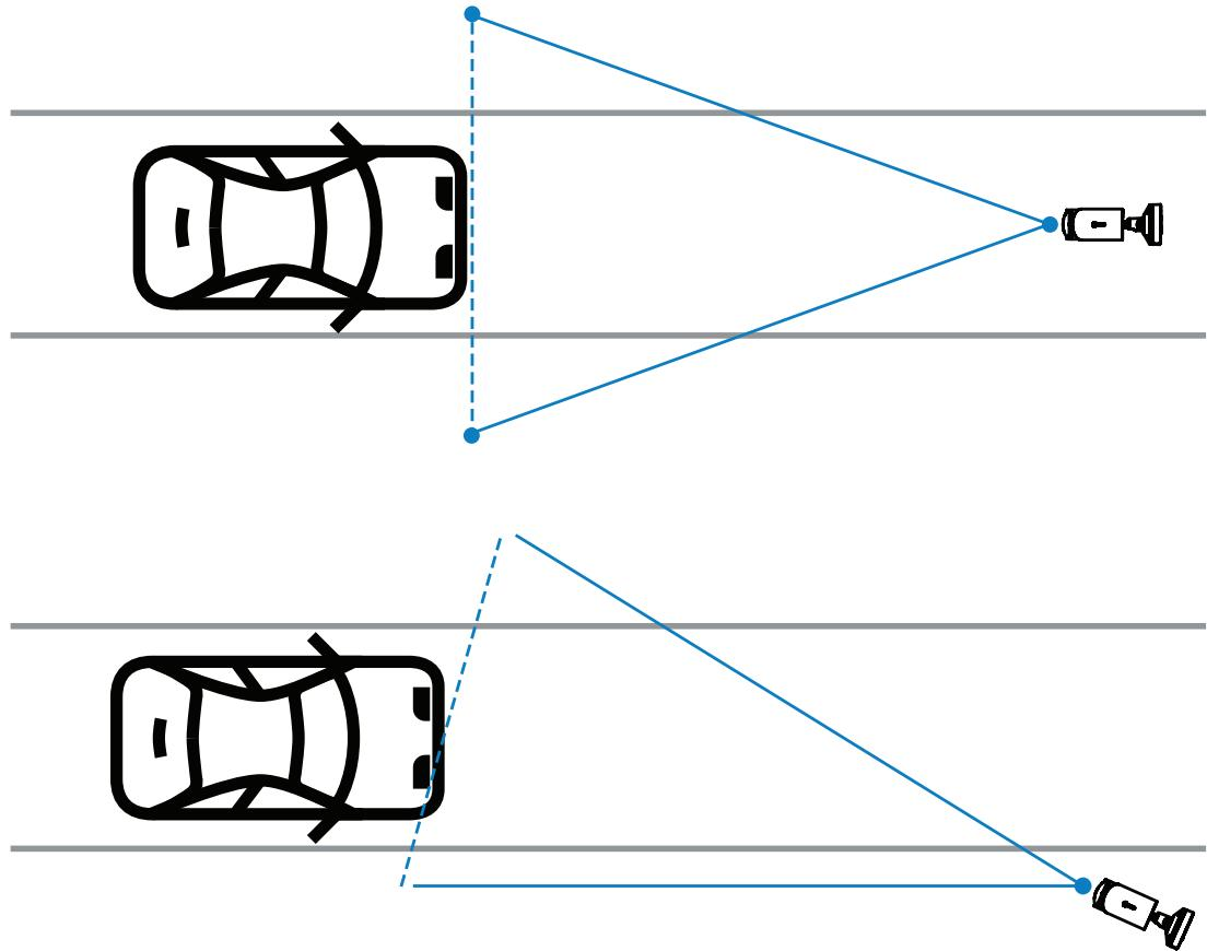
The field of view should be at least twice as wide as the lane to ensure that the front of the vehicle is visible.
