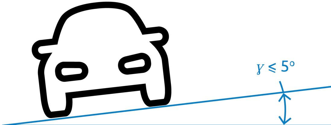
For best performance the tilt angle should be within the range of  $-5^\circ \leq \gamma \leq +5^\circ$ , but must be within the range  $-30^\circ \leq \gamma \leq +30^\circ$ .
